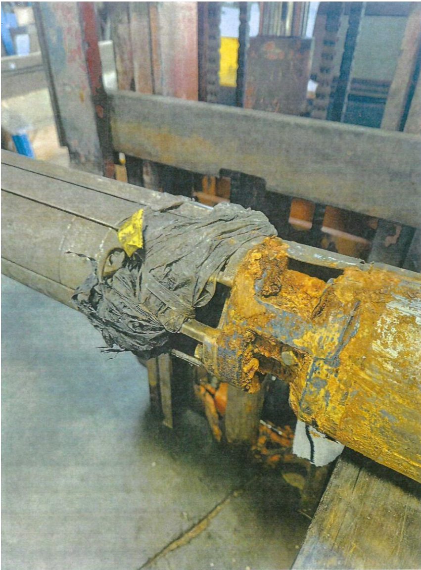
Plastic bags entwined in pump impeller.
